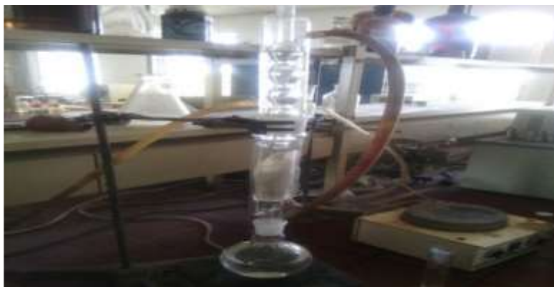
Figure 1: Soxhlet apparatus setup used for the oil extraction
